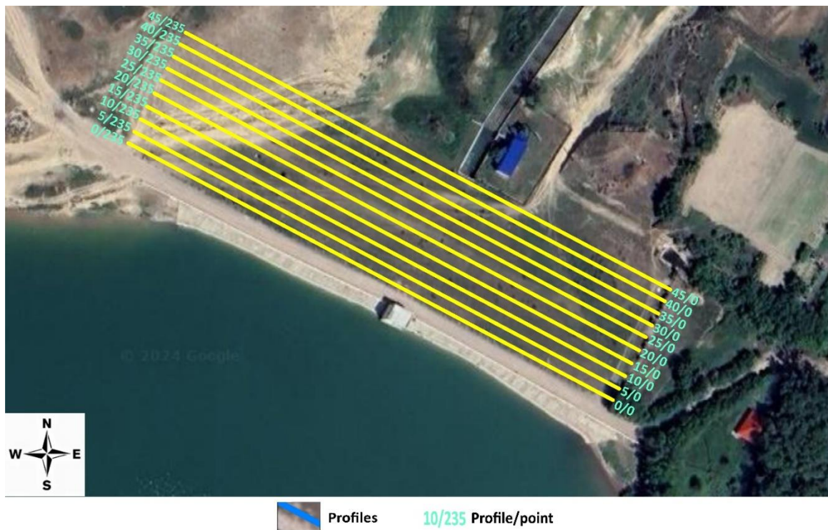
Figure 1. Scheme of the electrical resistivity tomography profiles.
