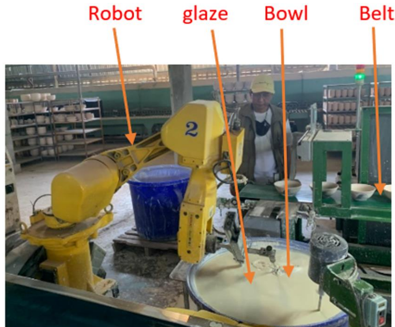
Figure 11. Ceramic bowl glazing that is automated (step 2).
