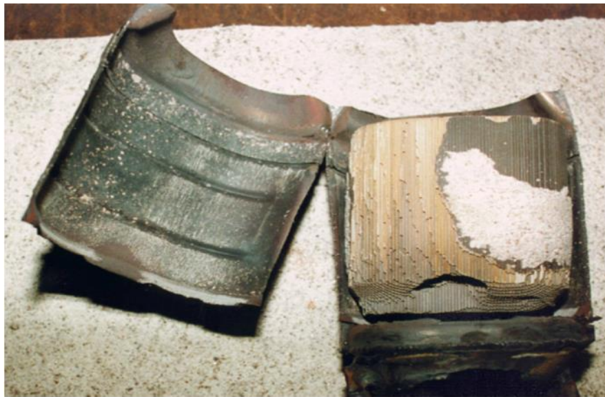
Figure 2. Substrate erosion caused by non-uniform flow [23].
