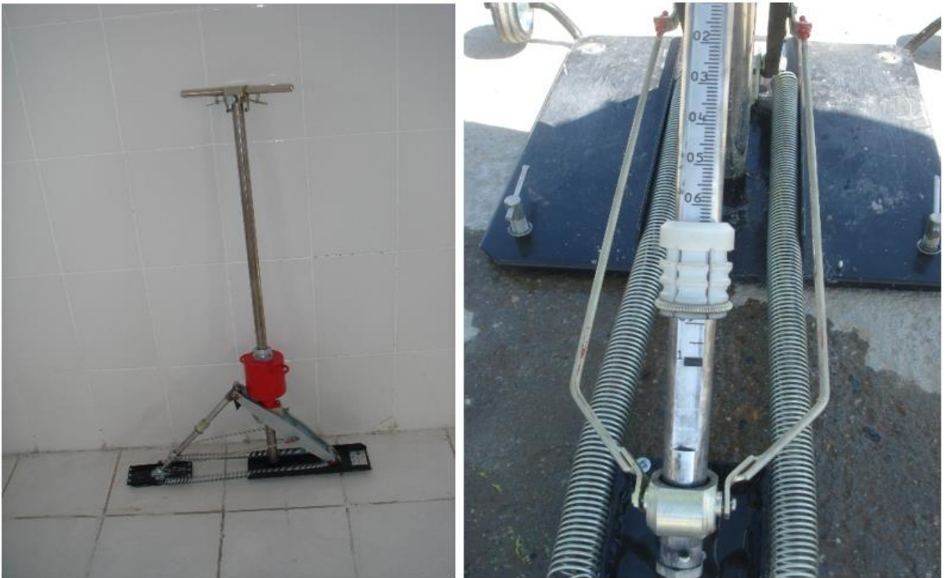
Figure 4. Portable device for measuring the friction coefficient named IKSp-M and the measurement process.
