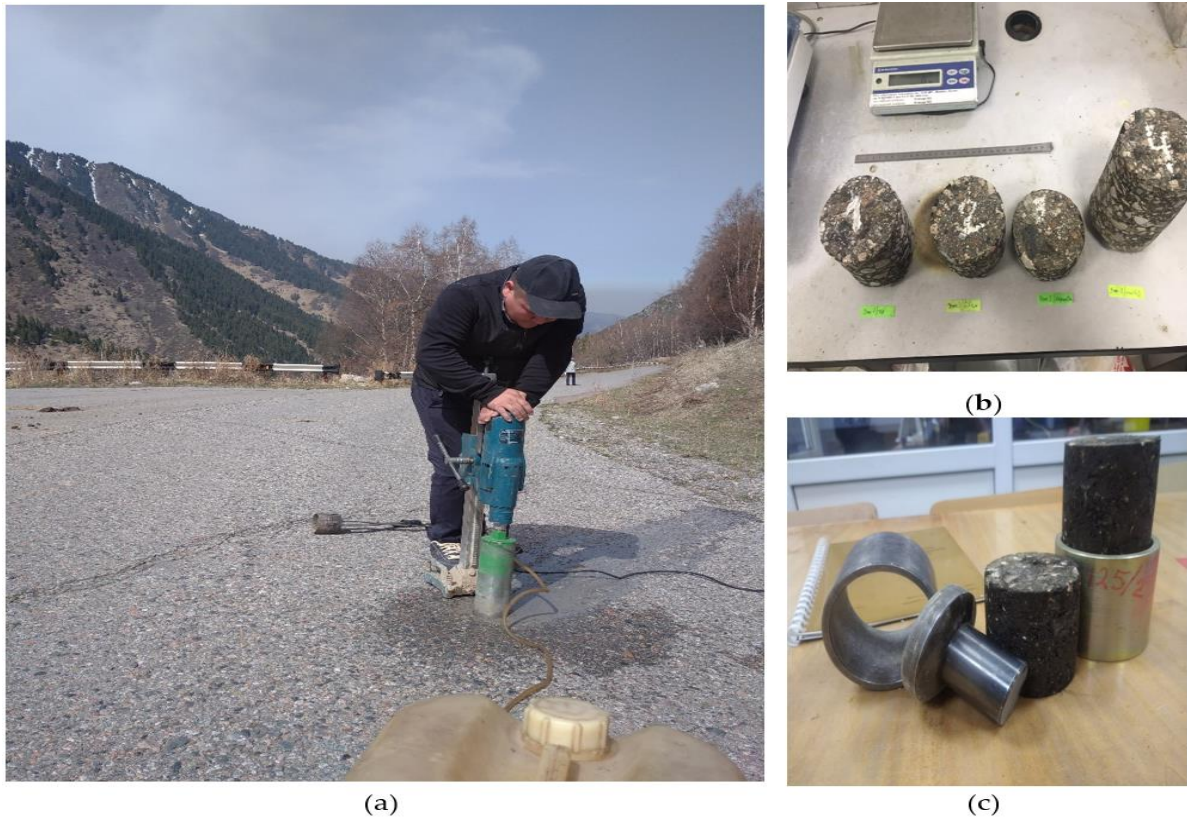
Figure 15. Asphalt concrete samples: (a) sampling in the field; (b) samples from 4 sections of the road under study; (c) reference materials prepared in the laboratory.
