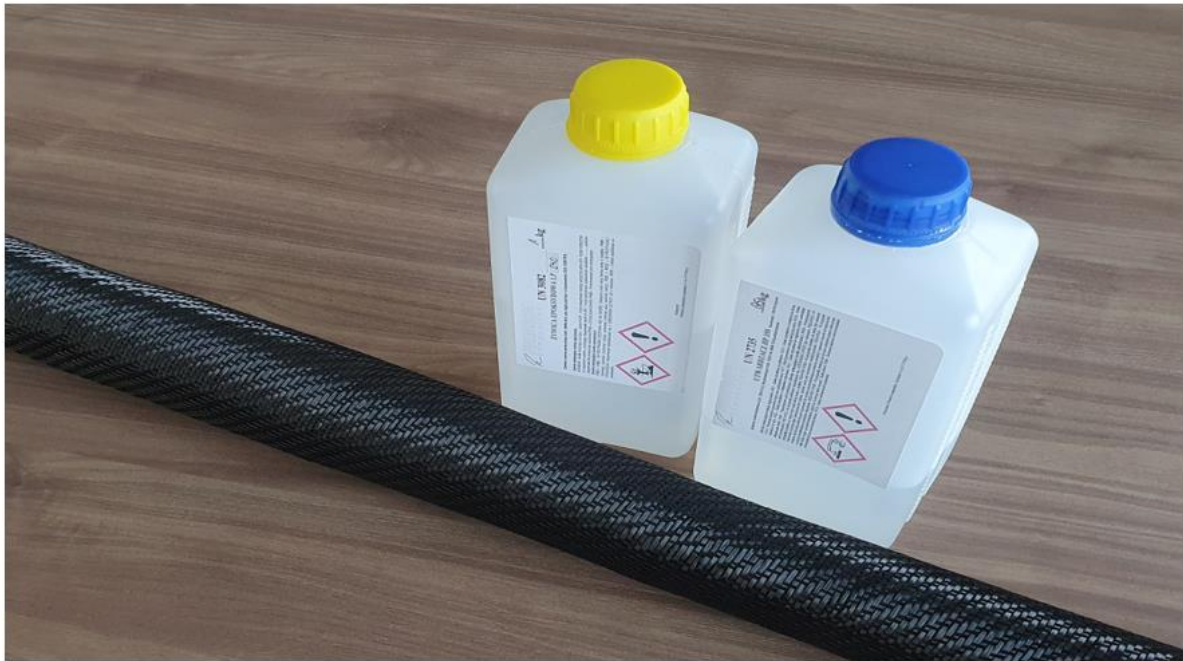
Figure 1. Carbon fabric and epoxy resin used to create control plates.
