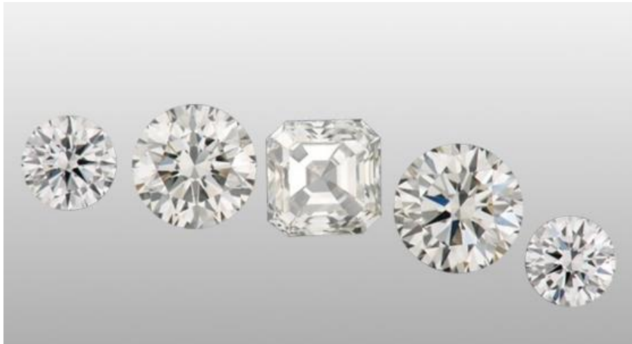
Figure 1. These synthetic diamonds are produced by chemical vapor deposition (CVD). Source: https://www.gia.edu/gem-synthetic
