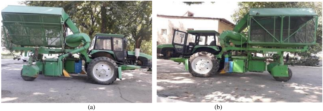
Figure 5. General view of the MX-1.8 GV cotton harvester with the standard (a) and newly developed (b) receiving chambers.
