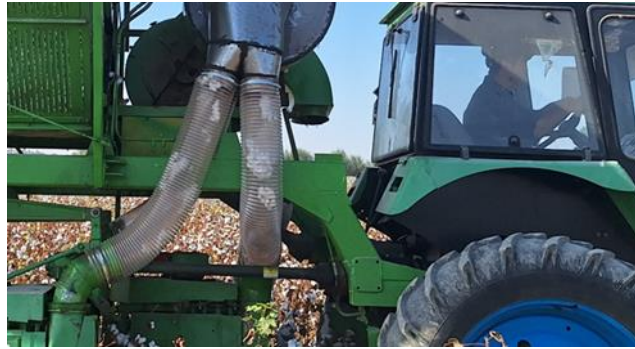
Figure 2. Raw cotton movement in a flexible transparent pipeline during machine harvesting
