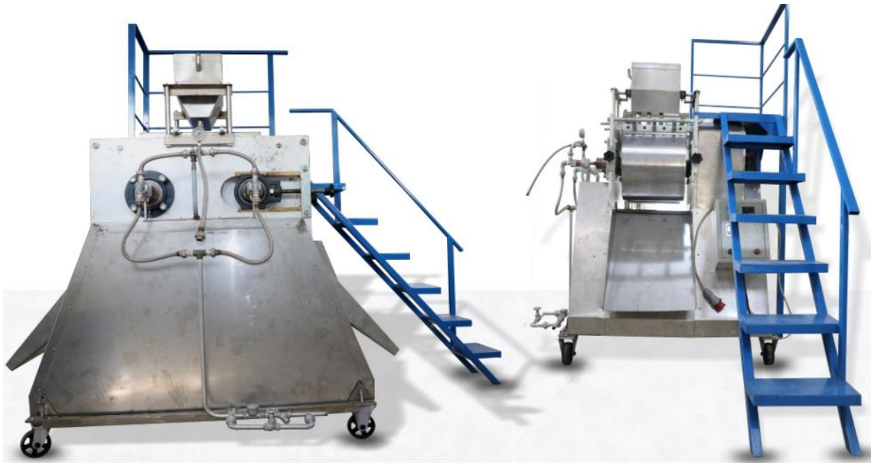
Figure 2. Drum dryer developed for pilot plant-scale instant slurry production.
