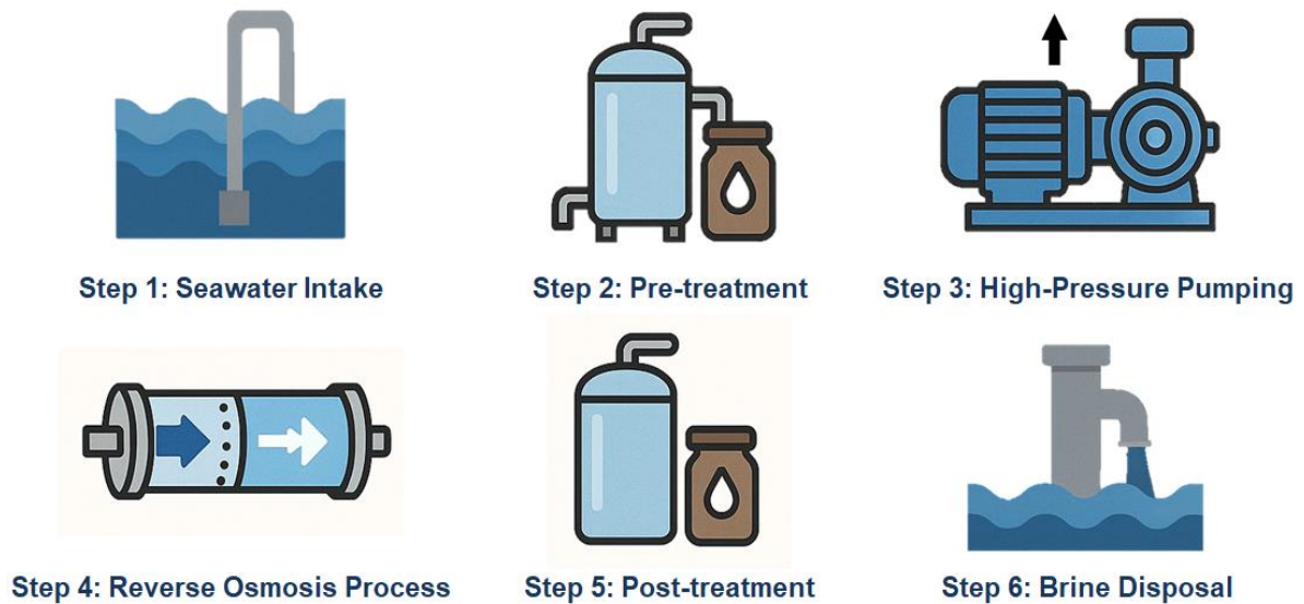
Figure 2. Steps Involved in Reverse Osmosis (RO) Process.
