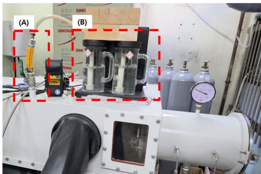
Figure 6. Gas exhaust assembly: (A) exhaust takeoff from the processing enclosure; (B) two-stage NaOH/BTB wet scrubber for neutralization and visual pH tracking prior to discharge.
