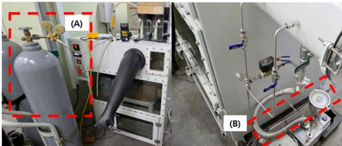
Figure 5. Argon (Ar) injection hardware: (A) supply and flow-control panel; (B) bottom-entry injection line to the processing section for uniform inerting under O_2 -sensor feedback control.
