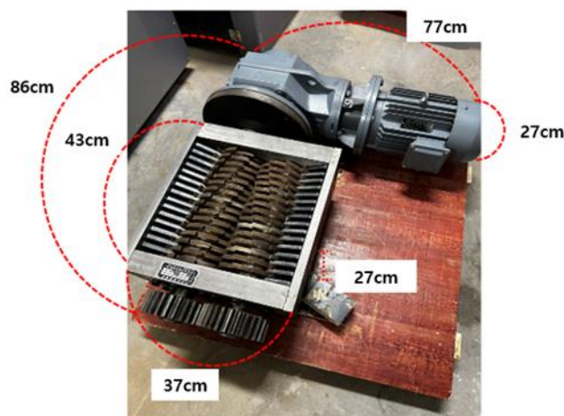
Figure 3. Integrated low-speed/high-torque shredder for spent lithium-ion batteries.
