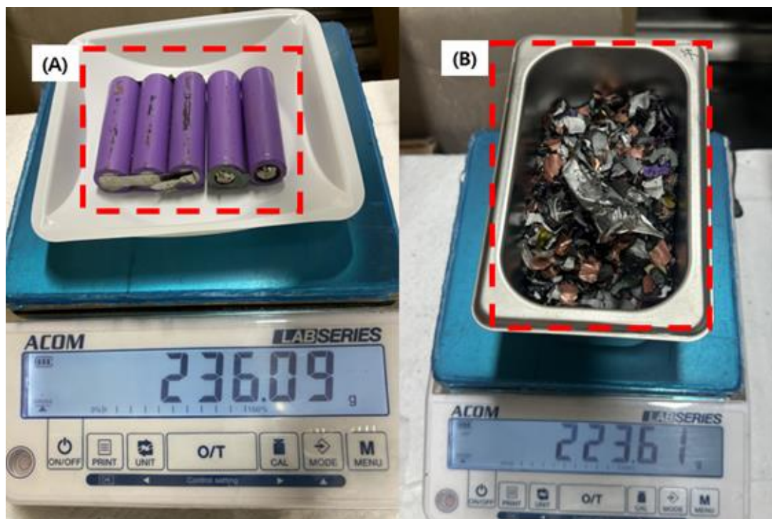
Figure 11. Spent cylindrical LIBs before and after treatment. (A) Five 18650 cells prior to shredding (batch mass 236.09 g) (B) Collected shredded solids after inert shredding and 300 °C drying (mass 223.61 g).
