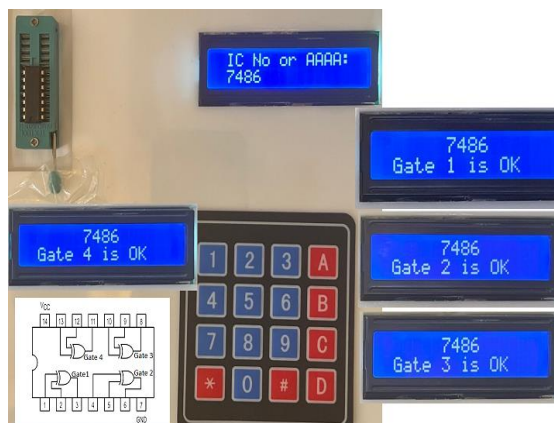
Figure 14. In the 7486 IC test, each of the four XOR gates operate as intended.
