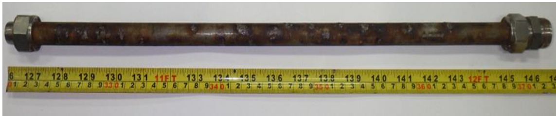
Figure 2. Visual examination of the failed tube (Location 1) reveals that the majority of the outer surface is covered by corrosion products.
