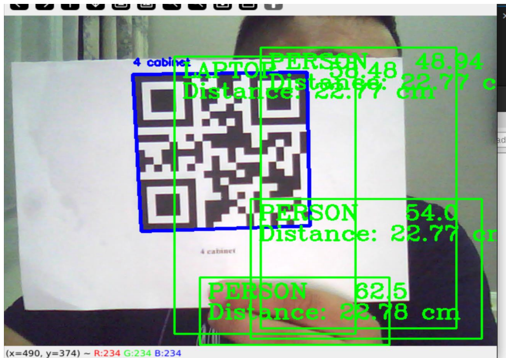
Figure 13. QR code recognition, object localization, and distance estimation process.
